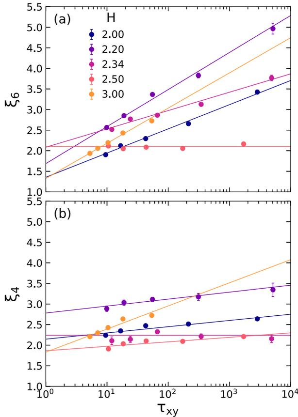
**Figure 6.** Correlation length scales associated with (a)  $\xi_6$  and (b)  $\xi_4$  for particles within the contact layers adjacent to the walls as a function of the in-plane relaxation time  $\tau_{xy}$ . The systems have polydispersity  $s = 0.15$  and wall separations  $H$  indicated in the legend. Solid lines are fits to the relation  $\tau_{xy} = B \exp(C \xi_i)$ , where  $B$  and  $C$  are positive constants and  $\xi_i$  is either  $\xi_4$  or  $\xi_6$ .
