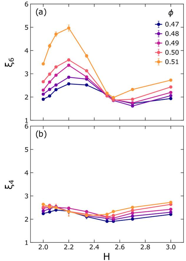
**Figure 5.** Correlation length scales associated with (a)  $\xi_6$  and (b)  $\xi_4$  for particles within the contact layers adjacent to the walls as a function of  $H$ . The systems have polydispersity  $s = 0.15$  and volume fractions  $\phi$  indicated in the legend. Error bars reflect uncertainties in  $\xi_l$  from fits of the peaks of  $g_l(r)/g(r)$  to decaying exponential functions (Equation (6)).
