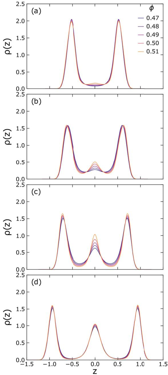
**Figure 2.** Number density profiles  $\rho(z)$  in the direction perpendicular to the confining walls for (a)  $H = 2.20$ , (b)  $H = 2.34$ , (c)  $H = 2.50$ , and (d)  $H = 3.00$  and volume fractions  $\phi$  denoted in the legend. Each system has a polydispersity of  $s = 0.15$ .
